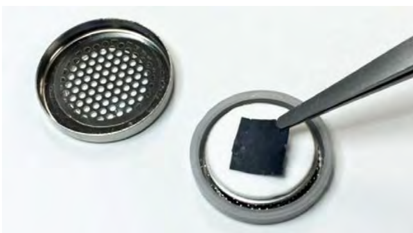
A nanoporous electrode made from graphene complexes can dramatically boost charge storage in 'breathable' lithium–oxygen batteries.
