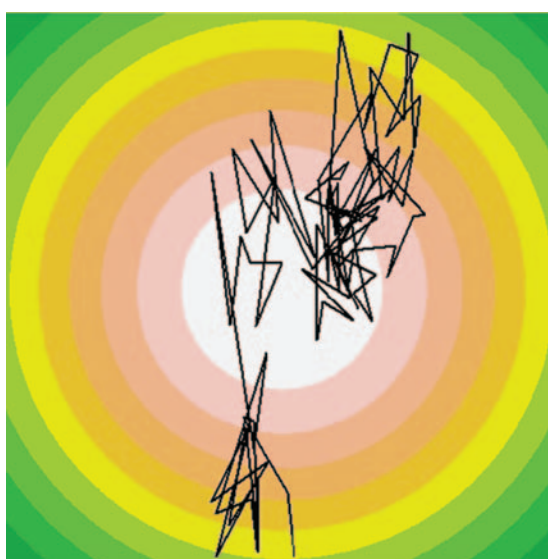
A representation of the combined mathematical and materials study into the deposition of electroactive thin films. The simulated trajectory of a lithium atom at an oxygen pressure of 10^{-6} torr (black line) is superimposed over a plot of a lithium plasma plume after expanding for 5 microseconds at an oxygen pressure of 10^{-2} torr (background).
