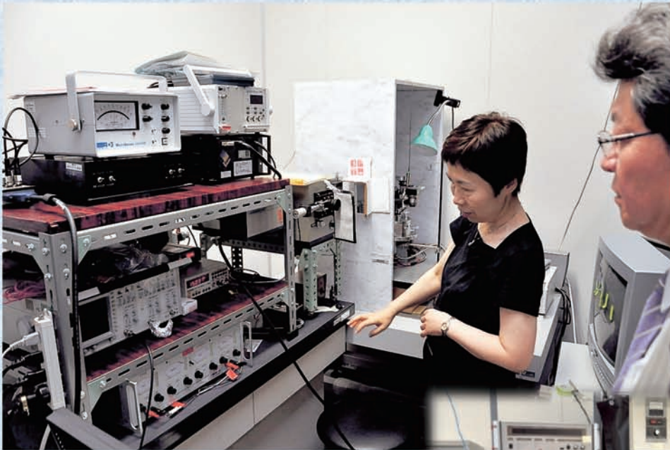
Surface Forces Apparatus and Resonance Shear Measurement System
