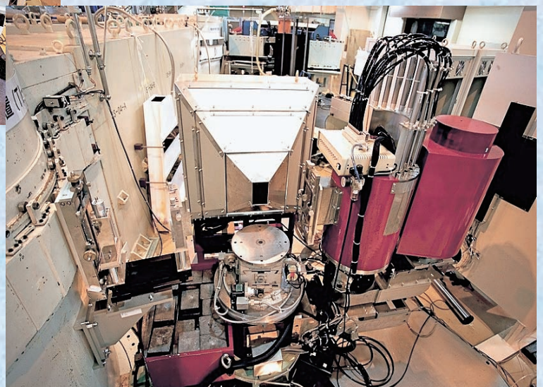
AKANE: Triple-Axis Neutron Spectrometer (JAEA)
