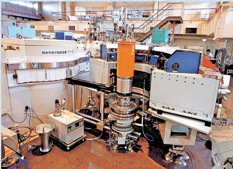
HERMES: Neutron Powder Diffractometer for High Efficiency and High Resolution Measurements (Japan Atomic Energy Agency (JAEA) in Ibaraki prefecture)
