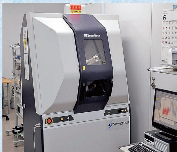
X-ray Diffraction System for Ultrathin Films
