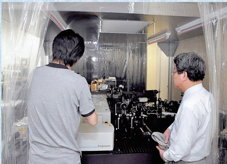
Time-Resolved Magneto-Optical Kerr Effect Measurement System for Spin Dynamics Investigation
