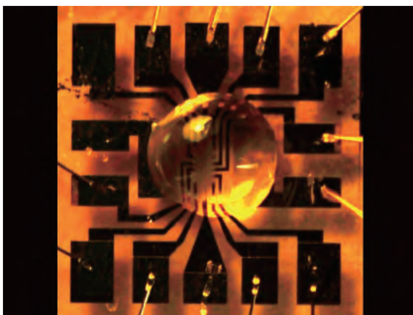
Photograph of the electric double layer transistor with a drop of ionic liquid for testing for superconductivity in KTaO 3
