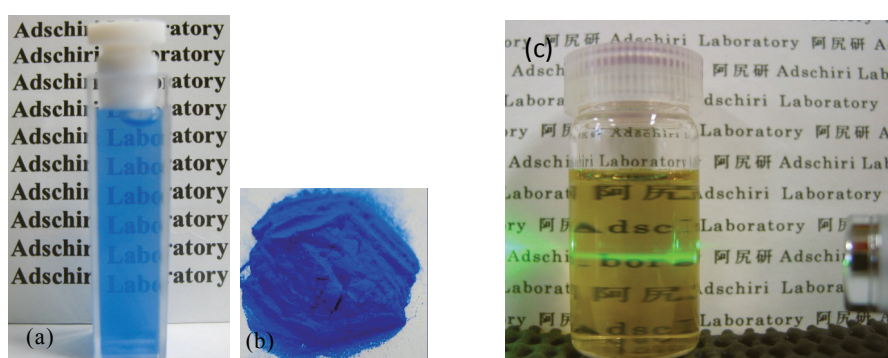
Figure 13. Perfect dispersion of CoAl 2 O 4 nanoparticles (b) in water (a) and CeO 2 nanoparticles in the organic solvent (c). Tyndall effect was clearly observed (c).
